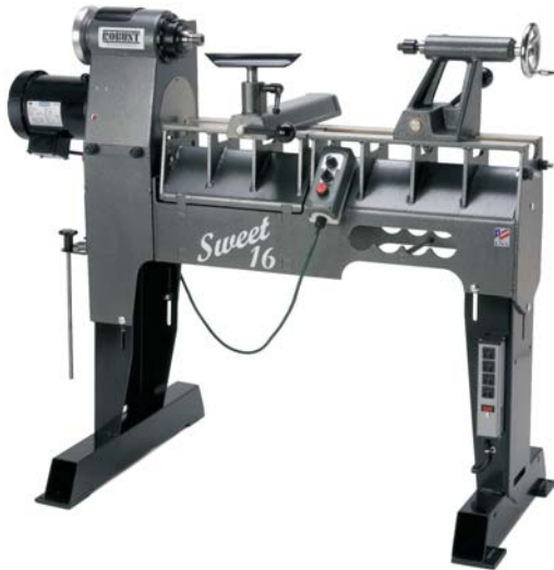
Above: Standard bed Sweet 16 as a normal 16" x 26" lathe.
